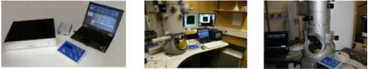
FIG. 4 (left to right) Digital precession unit DigiSTAR and its interface with FEI T30 FEG (Mainz, Germany) and Zeiss Libra 200 Cs corrected, Zeiss SMT Oberkochen, Germany
